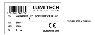
Maximum number of LED modules for daisy-chaining at driving current 80mA = 65 (in total for all luminaires)
