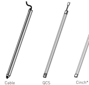
\*When using the Cinch luminaires it is recommended to use a strain relief to comply with EN 60335
