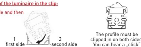
The profile must be clipped in on both sides!
